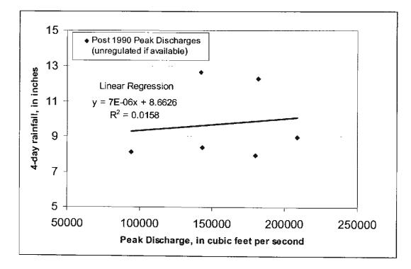
Figure 3. Post 1990 Peak Discharges on Skagit River near Concrete versus 4-day rainfall totals at Diablo, Washington.
