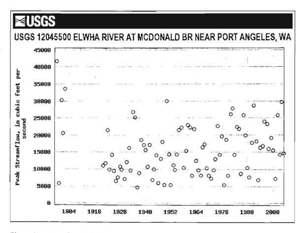
Figure 1a. Annual peak discharges recorded at the Elwha River at McDonalds Bridge near Port Angeles, Washington. The Elwha River has not been regulated for flood control.
