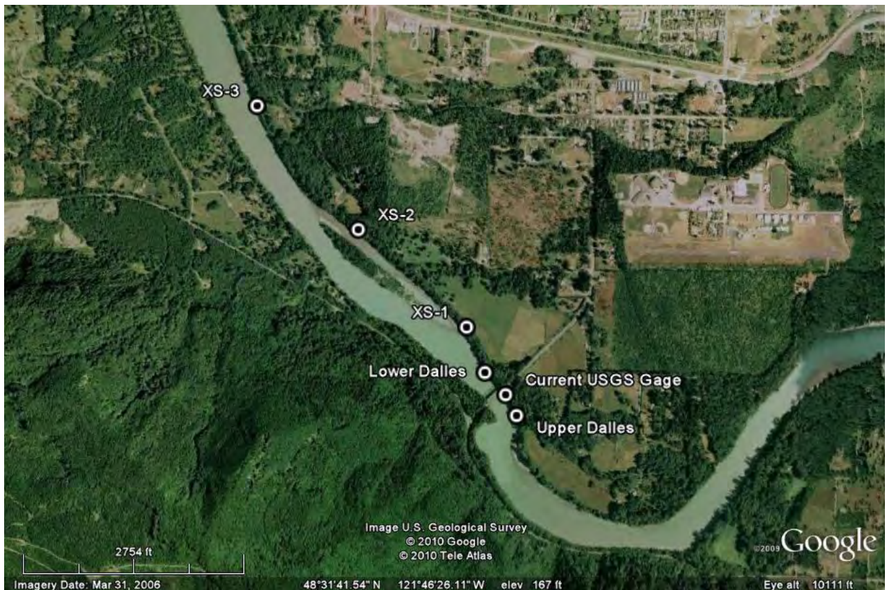
Aerial view of the Dalles gorge showing current and old gage locations and the locations of Stewart's slope-area cross sections XS1, XS2, and XS3.
