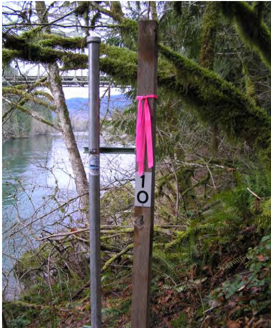
Skagit County Crest Stage Gage #10. Note the Dalles bridge 200 feet downstream. The current USGS gage is on the right bank just upstream of the bridge.
