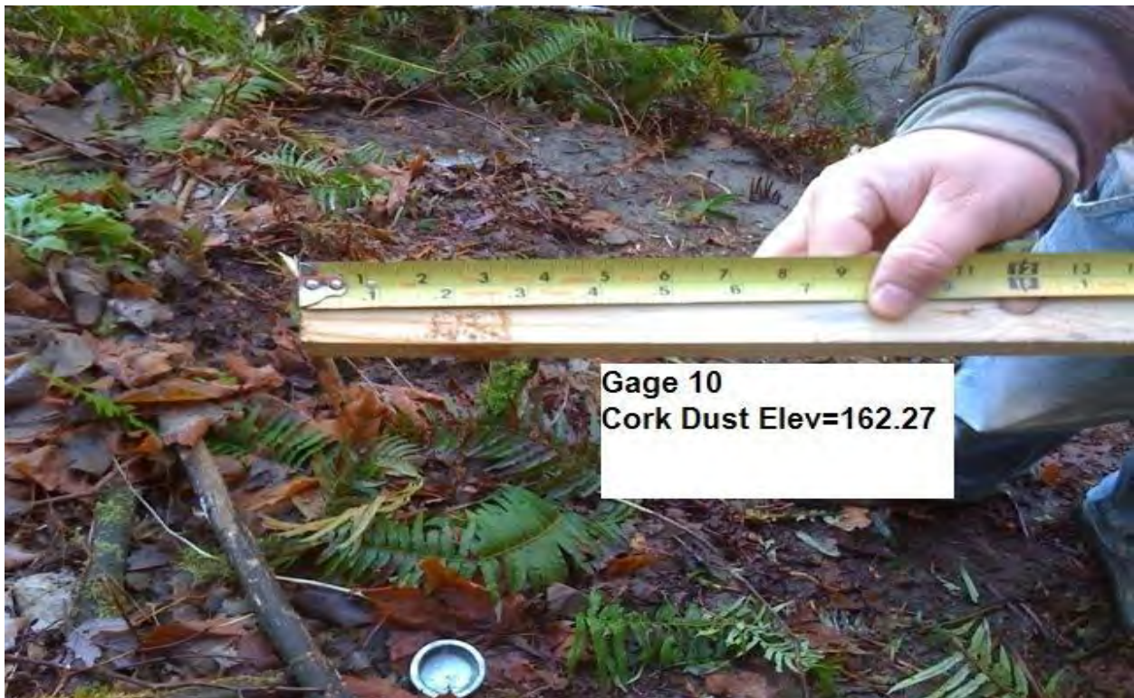
Photograph showing cork dust marks left on inside crest stage gage 200 feet upstream of the USGS Concrete gage at the Dalles, WA. December 2010.
