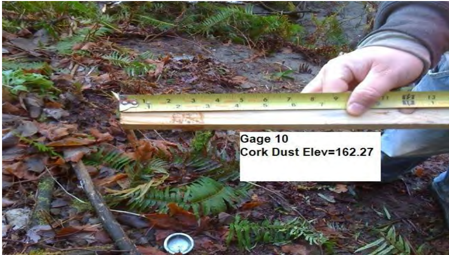
Photograph showing cork dust marks left on inside crest stage gage 200 feet upstream of the USGS Concrete gage at the Dalles, WA. December 2010.
