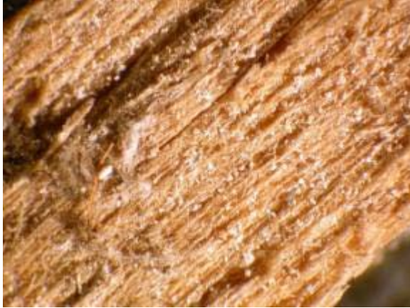
Figure 55. M-11 McManaman - Light deposits of dust to silt-size siliceous mineral grains and biological material. Magnification approximately 10X.
