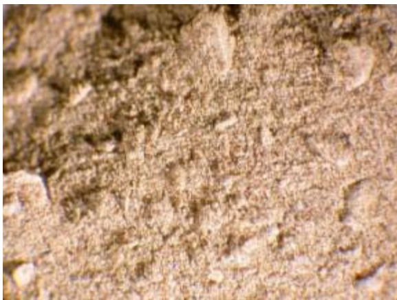
Figure 42. 45956 #1 Ripple No. 2 - Fine pale beige gray powder consisting of clay, insect parts, pollen, spores, minor quartz, feldspar, wollastonite, iron oxides, plant material, soot, traces of others. Magnification approximately 10X.
