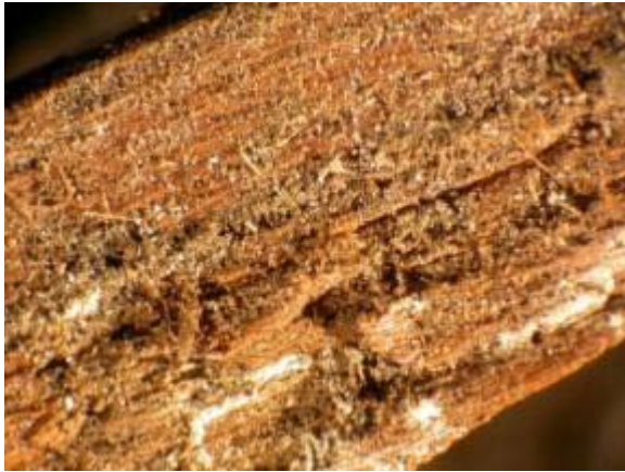
Figure 10. G-6 Gifford - Biological materials and light to moderate deposits of debris on wood surface. Magnification approximately 10X.
