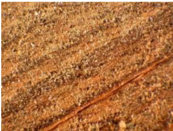
Figure 6. G-2 Gifford - Light to moderate deposits of mineral debris on wood surface. Magnification approximately 10X.
