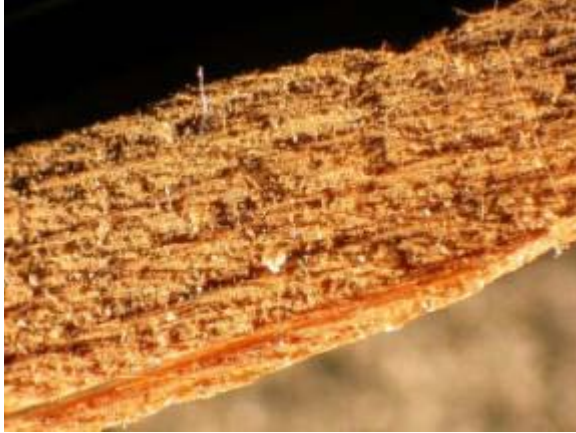
Figure 31. R-8 Ripple No. 1 - Light deposits of insect parts and other biological materials, traces of dust-size mineral grains. Magnification approximately 7X.
