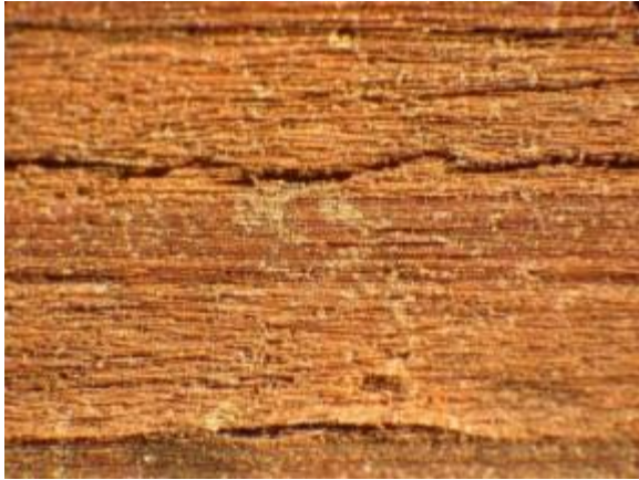
Figure 1. F-1 612 Fairhaven - Small amount of dust-size particles cling to the surface of the wood. Magnification approximately 10X.
