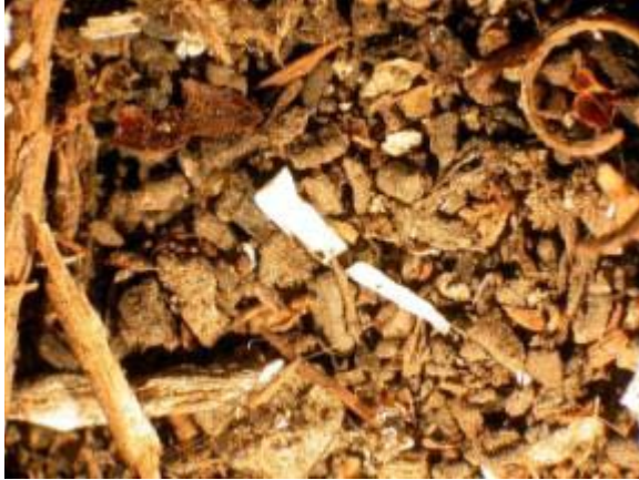
Figure 22. G-20 Gifford - Wood chips, paint flakes, insect casts, insect parts, plant fibers/rootlets, spider silk, rodent pellets, corrosion scale, siliceous mineral grains ranging from silt-size to coarser particles. Magnification approximately 10X.
