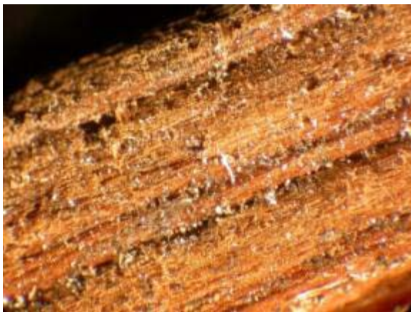
Figure 12. G-8 Gifford - Small amounts of silt-size particles and small amounts of biological material on wood surface. Magnification approximately 10X.
