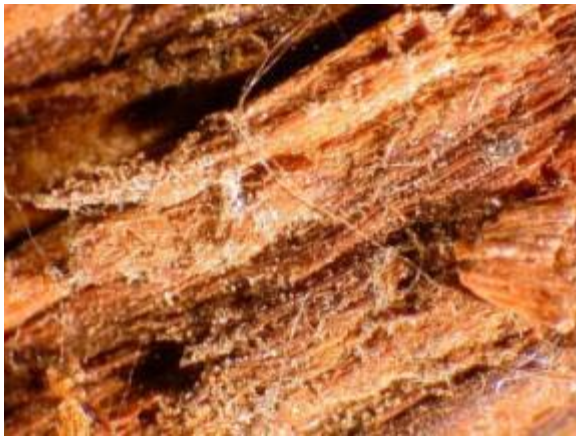
Figure 53. M-8 McManaman - Light deposits of dust to silt-size siliceous mineral grains, insect parts, and fibrous biological material. Magnification approximately 15X.
