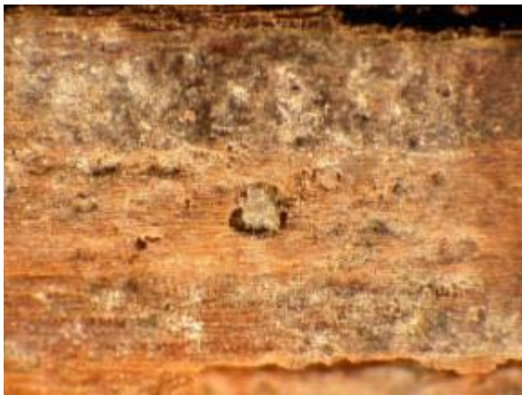
Figure 2. F-2 612 Fairhaven - Locally heavy deposits on wood surface. Magnification approximately 10X.
