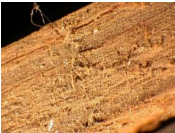
Figure 33. R-10 Ripple No. 1 - Moderate deposits of dust-size mineral grains, insect part and other biological materials. Magnification approximately 10X.
