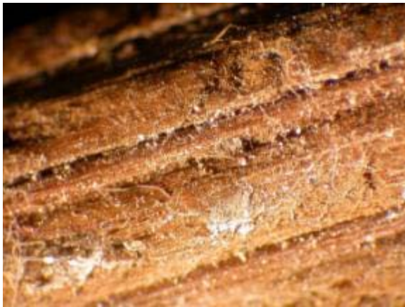
Figure 17. G-14 Gifford - Light deposits of silt-size mineral deposits and small amounts of biological materials on wood surface. Magnification approximately 15X.
