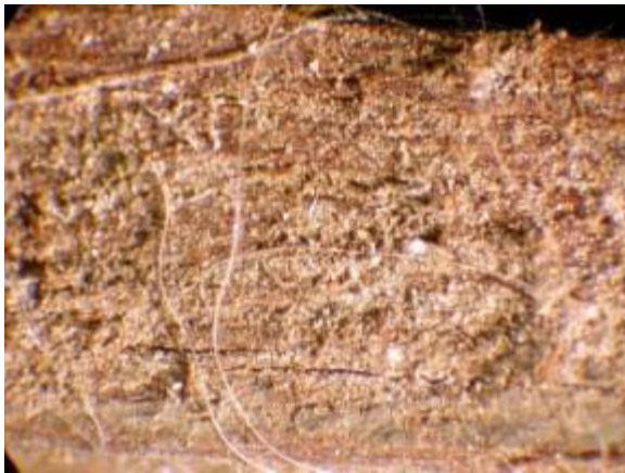
Figure 47. M-2 McManaman - Heavy deposits of silt-size siliceous mineral grains, smaller amounts of biological material (much is fibrous). Magnification approximately 10X.
