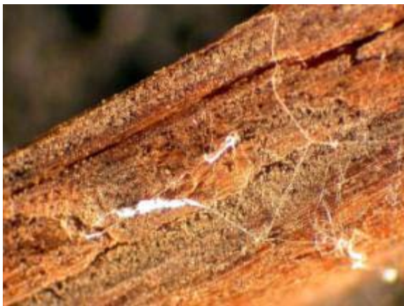
Figure 18. G-15 Gifford - Light deposits of silt-size mineral deposits, spider silk and dark biological materials on wood surface. Magnification approximately 10X.
