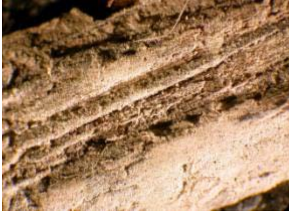
Figure 13. G-10 Gifford - Very heavy deposits of silt-size mineral deposits, possibly cementitious material, and small amounts of biological materials on wood surface. Magnification approximately 10X.
