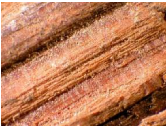
Figure 51. M-6 McManaman - Light deposits of dust and silt-size siliceous mineral grains, mostly in crevices. Locally, fibrous biological materials and insect parts. Magnification approximately 15X.
