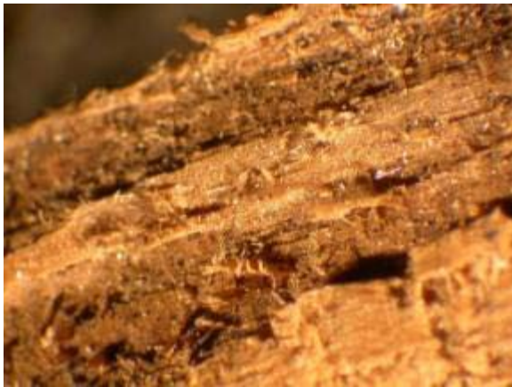
Figure 8. G-4 Gifford - Dark biological materials and light deposits of debris on wood surface. Magnification approximately 10X.
