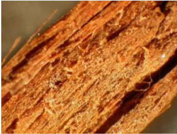
Figure 28. R-5 Ripple No. 1 - Traces of dust to silt-size mineral grains and biological materials. Magnification approximately 10X.
