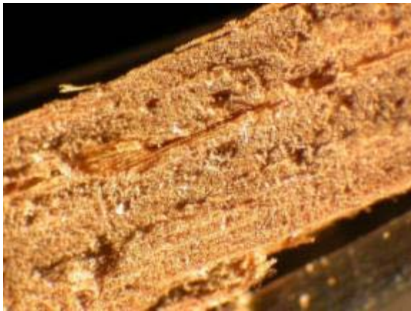
Figure 29. R-6 Ripple No. 1 - Moderate deposits of insect parts and other biological materials, traces of dust-size mineral grains. Magnification approximately 10X.
