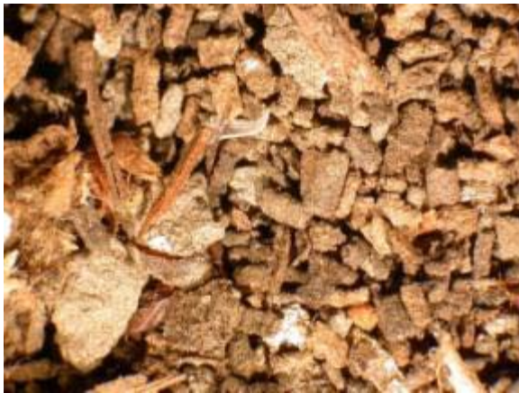
Figure 23. D-10 Ripple No. 1 - Wood fragments, insect parts, rodent fecal pellets, various plant debris, small amounts of siliceous minerals (mostly coarse), paint flakes, and mortar. Magnification approximately 10X.
