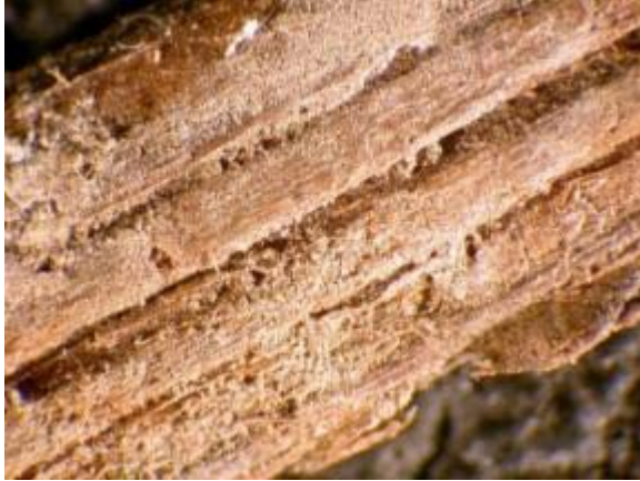
Figure 16. G-13 Gifford - Light to locally heavy deposits of silt-size mineral deposits and small amounts of biological materials on wood surface. Magnification approximately 10X.
