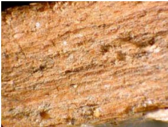
Figure 57. M-13 McManaman - Trace deposits of dust-size siliceous mineral grains and biological material. Magnification approximately 10X.
