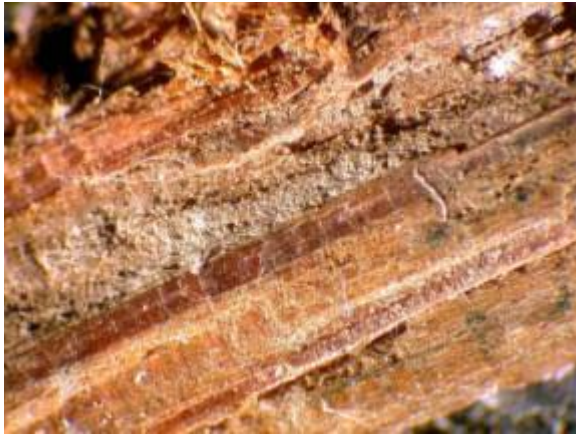
Figure 19. G-16 Gifford - Light deposits of silt-size mineral deposits and small amounts of biological materials on wood surface. Magnification approximately 15X.
