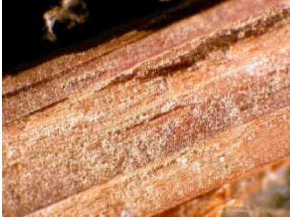
Figure 52. M-7 McManaman - Light deposits of dust to silt-size siliceous mineral grains and fibrous biological material. Magnification approximately 10X.
