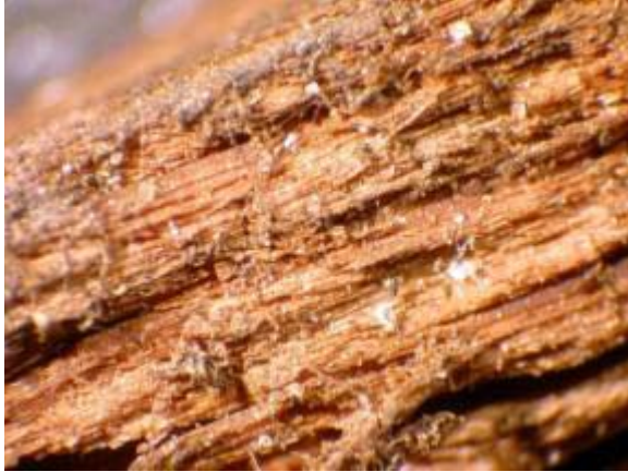
Figure 37. S-1 Ripple No. 2 - Light deposits of silt-size siliceous mineral grains and biological material. Magnification approximately 10X.
