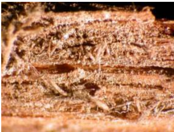
Figure 48. M-3 McManaman - Moderate deposits of silt-size siliceous mineral grains, insect parts, and other biological materials. Magnification approximately 10X.
