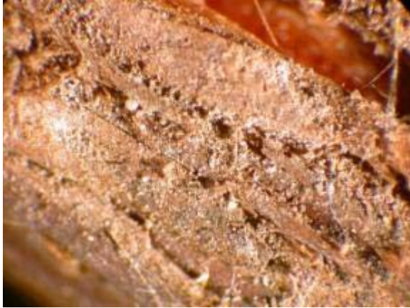
Figure 49. M-4 McManaman - Light to moderate deposits of dust to silt-size siliceous mineral grains and biological material. Magnification approximately 10X.
