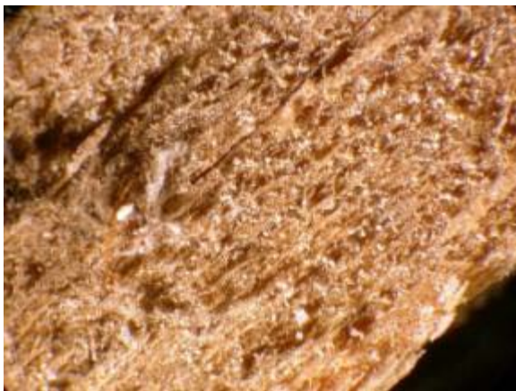
Figure 54. M-10 McManaman - Light to moderate deposits of dust to silt-size siliceous mineral grains, insect parts, and biological material. Magnification approximately 15X.
