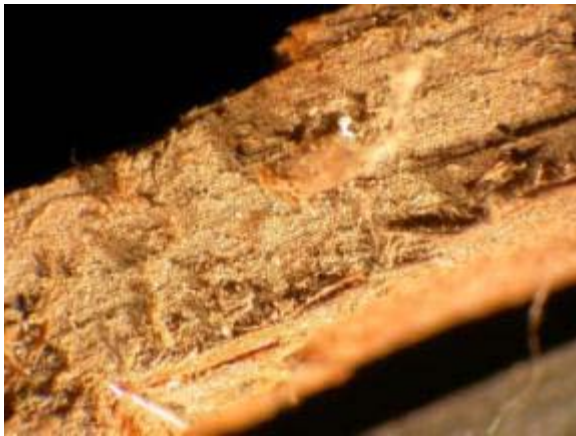
Figure 35. R-12 Ripple No. 1 - Moderate deposits of dust-size mineral grains, insect part and other biological materials. Magnification approximately 7X.
