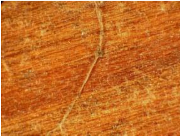
Figure 4. F-4 612 Fairhaven - Traces of dust-size particles and small amounts of biological materials on wood surface. Magnification approximately 10X.
