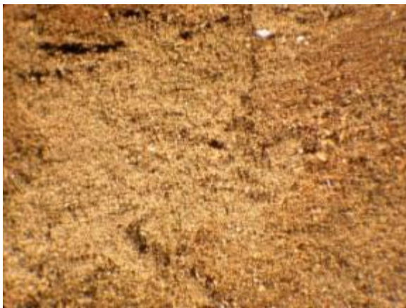
Figure 24. R-1 Ripple No. 1 - Heavy deposits of silt-size siliceous mineral grains, insect parts, and other biological materials. Magnification approximately 10X.
