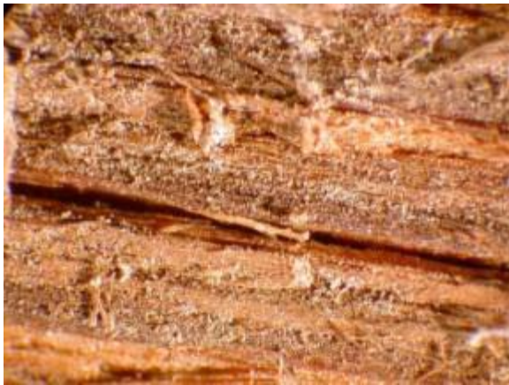
Figure 50. M-5 McManaman - Light to moderate deposits of dust to silt-size siliceous mineral grains and biological material. Magnification approximately 10X.
