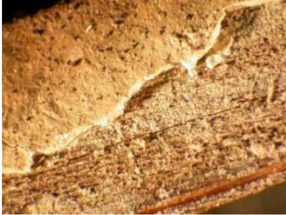
Figure 7. G-3 Gifford - Caulk and light deposits of debris on wood surface. Magnification approximately 10X.
