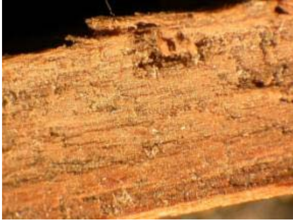
Figure 34. R-11 Ripple No. 1 - Moderate deposits of dust-size mineral grains, insect part and other biological materials. Magnification approximately 10X.
