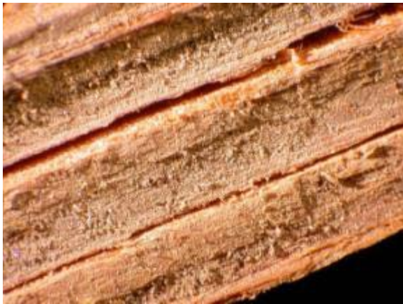
Figure 41. S-5 Ripple No. 2 - Light deposits of biological materials, traces of dust-size mineral grains. Magnification approximately 10X.
