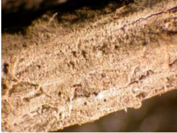
Figure 14. G-11 Gifford - Heavy deposits of silt-size mineral deposits, possibly cementitious material, and traces of biological materials on wood surface. Magnification approximately 10X.
