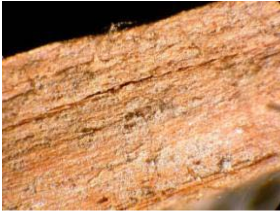
Figure 58. M-14 McManaman - Light deposits of dust to silt-size siliceous mineral grains and biological material. Magnification approximately 10X
