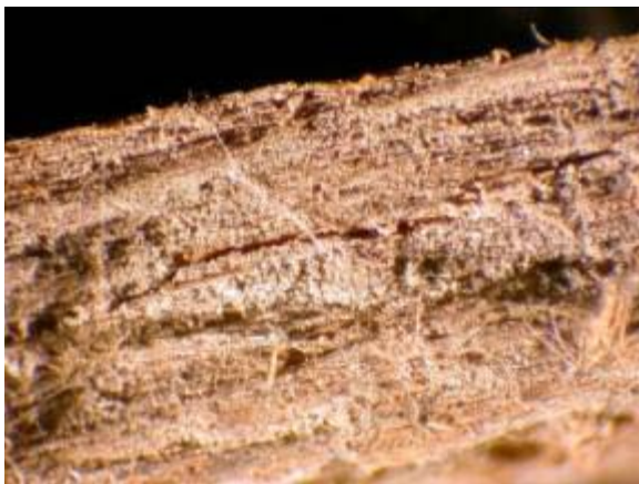
Figure 21. G-18 Gifford - Moderate to heavy deposits of silt-size mineral deposits and small amounts of biological materials on wood surface. Magnification approximately 10X.
