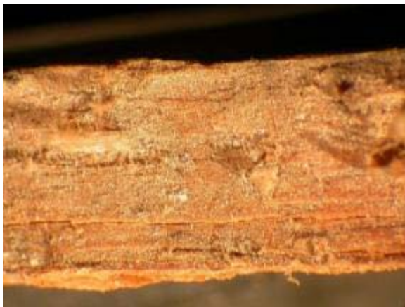
Figure 36. R-13 Ripple No. 1 - Light deposits of dust to silt-size mineral grains and small amounts of biological materials. Magnification approximately 7X.
