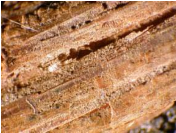
Figure 20. G-17 Gifford - Light deposits of silt-size mineral deposits and small amounts of biological materials on wood surface. Magnification approximately 15X.
