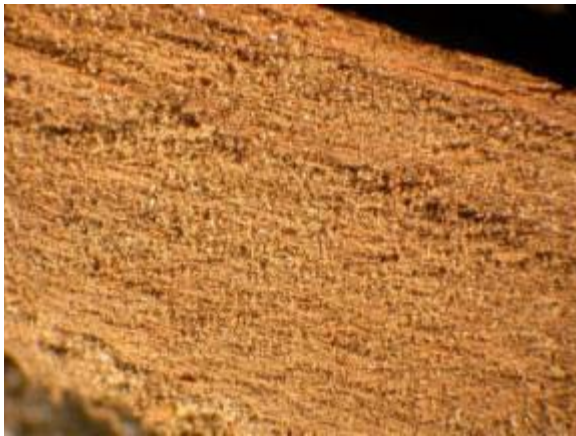
Figure 26. R-3 Ripple No. 1 - Moderate to heavy deposits of silt-size siliceous mineral grains, insect parts, and other biological materials. Magnification approximately 10X.
