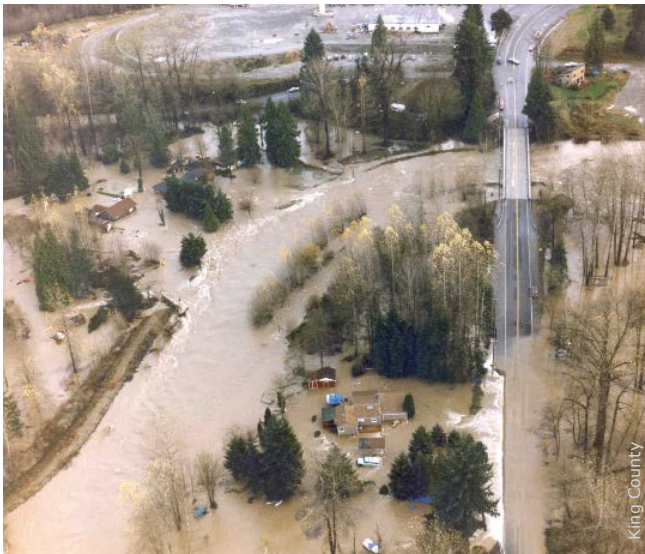
When levees fail, the results can be devastating. This photo shows a large section of levee washed out along the Cedar River during a 1990 flood.
