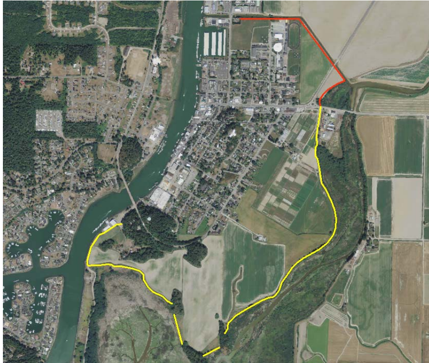
Figure 36: La Conner community levee (Orange line shows proposed alignment; yellow line shows existing levee)
