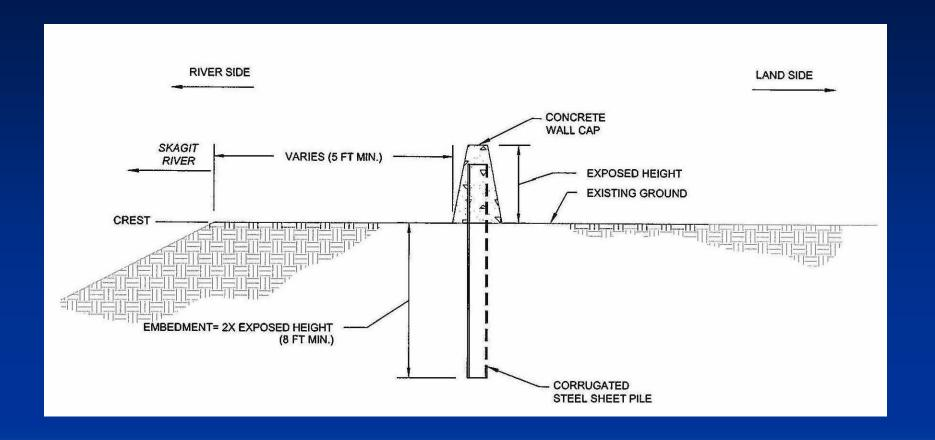
Typical Cantilever Sheet Pile Flood Wall Design
