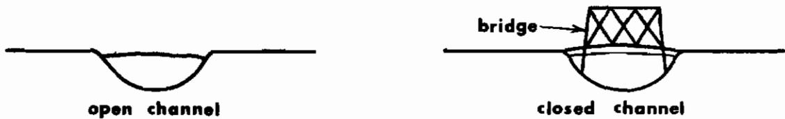
With a closed channel, only about 80 percent of an open channel flow can be handled because of top drag. (Howard Copp, ASCE, "Pullman Tackles Its Flooding Problems," Civil Engineering - ASCE, August 1972, p. 45)
