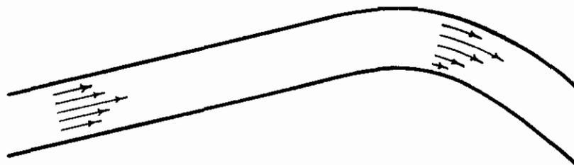
Thus, a transfer of force is exerted from the center of the river to the outside bank, which could create bank erosion and dike failures.
