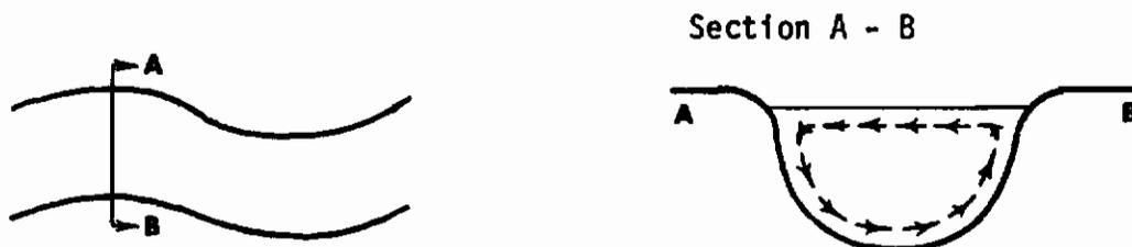
From this illustration, one can see that bedload materials (rocks, etc., that are dragged across the bottom) is eroded from the outer bank (A) to the inner bank (B).
