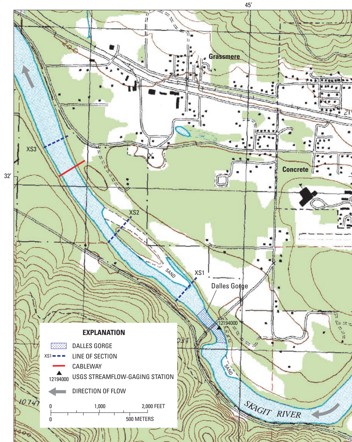
Figure 1. Location of cross sections, discharge measurement cableway, Dalles Gorge, and streamflow-gaging station Skagit River near Concrete, Washington.
