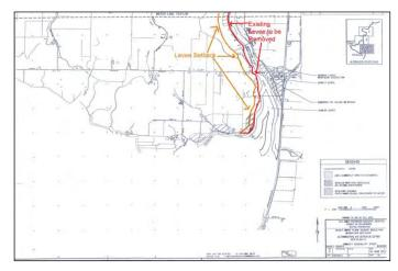
the difficulty in raising a levee on only one side of the river. In addition, the measure would require property purchased for a wider levee footprint and replacing large portion of existing infrastructure.
