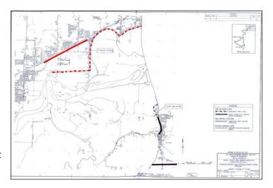
There were two designs for this levee developed in 2001 that are shown in the picture above. One of them ties in the levee at the upstream side at Sedro-Woolley and the downstream side at the existing levee system. It also encompasses most of the houses that are found in this area. The other design raises the ground elevation for the low spot only to match what is upstream and downstream.
