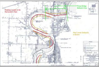
17.56 to 16.8. The setback starts at the top of bank elevation and the levee is moved back 500 feet from where it currently is. The setback alternates which side of the bank it is on based on a preliminary look at where the real estate would be cheaper to obtain. This layout is as follows:
